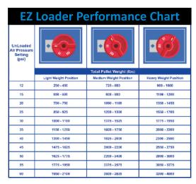
Based on a standard EZ Loader with rotator ring and no options. Addition of solid tops, etc will vary the PSI req.
